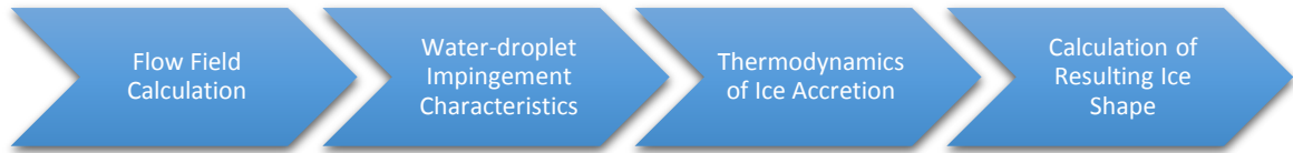
Figure 4: The four distinct modules incorporated within ice accretion solvers
