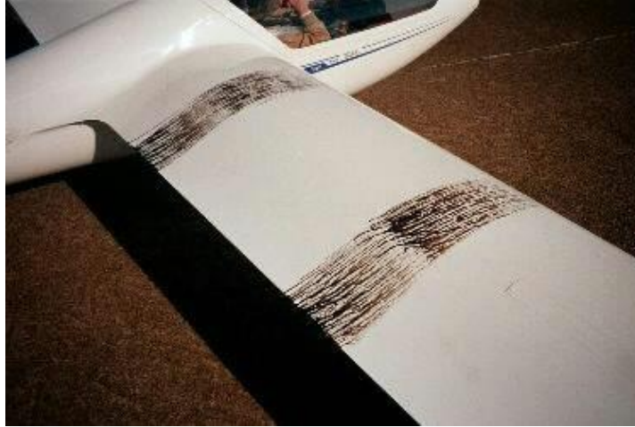
Figure 18: Flow visualization for a straight wing aircraft [41]
